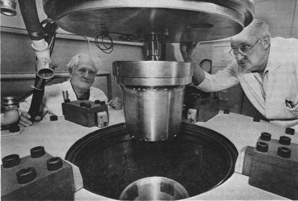
GARY SWAGERTY (right) and Dick Terwilliger lower a 200-lb. W79 test package into an air-driven spinner, where it will rotate at speeds up to 10,000 rpm — a rotation speed similar to the one a 155-mm artillery shell would experience when fired from a gun barrel. The spinner's maximum capability is 25,000 rpm.
